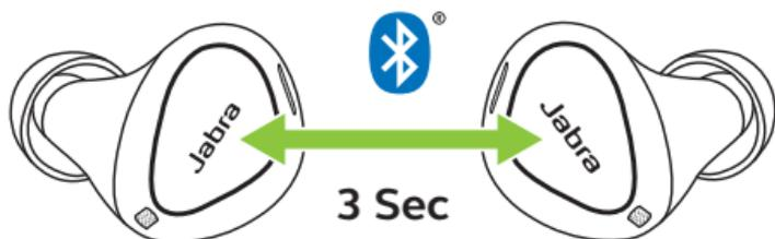
1. Power on the earbuds by removing them from the charging case. Alternatively, press the **Left** and **Right** buttons to power the earbuds on.
