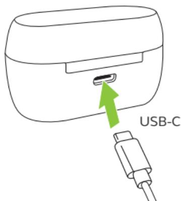
It is recommended to use a power supply with 5V  $\pm$ 0.25V and maximum charging current below 2A. It is not recommended to charge the earbuds or charging case using a wall charger with a higher voltage.
