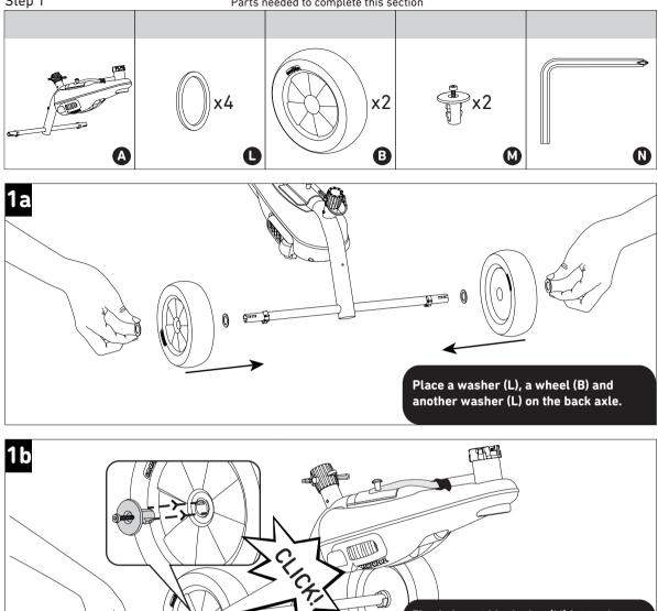
Firmly insert black plug (M) into axle opening, as shown. Align spring lock with dropout hole in axle and push firmly into position, until piece "clicks" into place.
