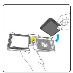
Remove the filters from the filter assembly.
