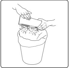
Tap the filter assembly over a wastebasket to remove any loose dust.
