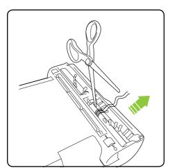
Carefully pull any hair or fibre from the brush bar. If you need to, you can slide a pair of scissors along the ridge in the brush bar.
