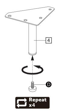
After fully assembled, part D can be loosen to make the unit stable on uneven floor.
