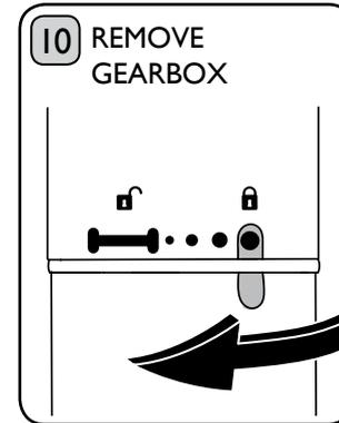
Remove the gearbox from the main body by twisting anti-clockwise.
