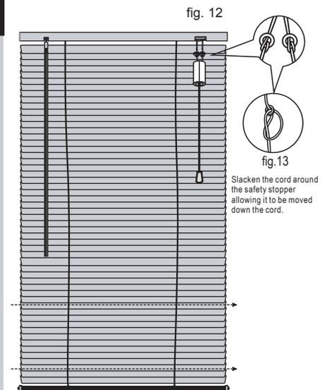
Slacken the cord around the safety stopper allowing it to be moved down the cord.
