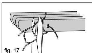
7. Knot lift cord directly beneath caps and cut off excess cord. Allow one extra rung and cut off excess ladder, now tuck remaining ladder into the bottom end slat cap holes. Replace caps. See fig. 17 and 18.
