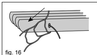
6. Remember to allow for the bottom end slat to be reinserted. Reinsert the lift cord through the cap holes and then insert back through the top and the caps. See fig. 17.
