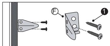
9. Hole on end cap of the bottom rail fits into Hold Down Brackets ❺ at the end of the window. See fig. 11.
