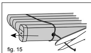
5. Count the number of slats you wish to remove. Pull lift cord from these slats to allow them to slide out of the ladder rung. See fig. 16.
