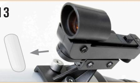
There is a small clear plastic tab inserted between the battery and the contact. This was included to prevent the battery from discharging during shipment. Pull this out to allow your battery to work.
