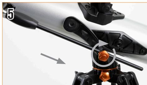
The altitude slow motion rod has a limited range of motion of about 15 degrees. If you run into the end of travel and the knob will no longer turn, you can reset it by loosening the rod guide knob and turning the slow motion rod handle the opposite direction until you are in the middle of its travel, then retighten the rod guide knob.
