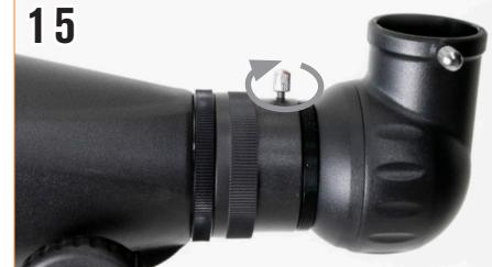
Insert the smaller tube on the diagonal into the back of the focuser and secure it by tightening the setscrews.
