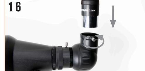
To install the eyepiece, loosen the setscrews on the open end of the star diagonal. Insert the silver barrel on the bottom of the eyepiece into the star diagonal and secure by tightening the setscrews. Always start using your low-power eyepiece (25 mm) to help you find the target you wish to view. You can always change to your high-power eyepiece (10 mm) later.
