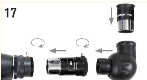
To use the Barlow lens, remove your star diagonal from the telescope, insert the Barlow lens into the telescope and insert your star diagonal into the Barlow lens. This will double the magnification of whatever eyepiece you use it with.
