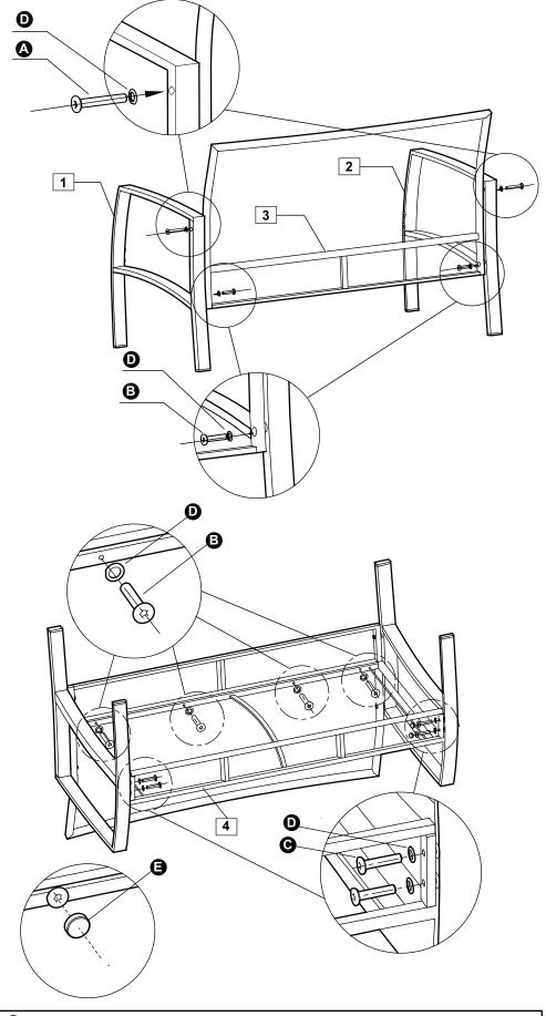
Important: Do not fully tighten all screws until assembly is complete.
