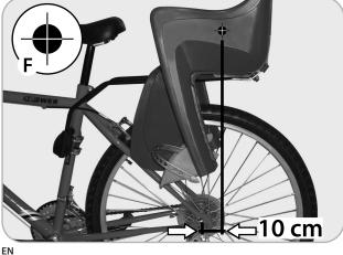
The seat has a gravity centre (F) (engraved on the seat) which cannot be more than 10cm away from the axle of the rear wheel. In case the gravity centre is at a longer distance, position the seat in another of the available positions (go back to page 9). Pay attention to the positioning of the seat; it must be adjusted so that the cyclist does not touch the seat when pedaling.
