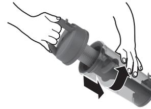
Turn the dust container lid anti-clockwise to unlock and lift to take out.
