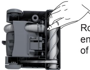
Rotate the brush to ensure free movement of the belt.
