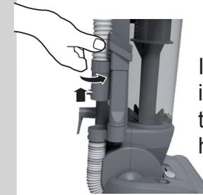
If cleaning tools were in use, check cleaning tool. Next check hose handgrip.
