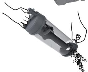
Hold the container over a bin and push the easy open button placed at the rear of the dust container.
