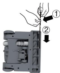
2 If you decide to fit wiper blade, then grip the side of the wiper blade and slide along the slot until the wiper blade is fully located. To disassemble, lift the end of the wiper blade and pull it out.
