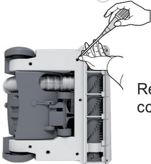
Remove the screws completely.
