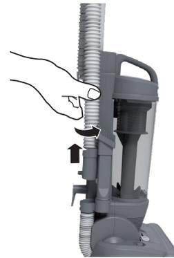
Attach crevice tool to the hose end connector.
