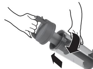
Whilst holding the lower part to lock together and twist the bin lid
