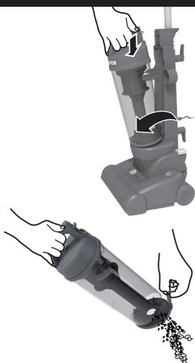
To remove the dust container from the cleaner, press the bin release button.
