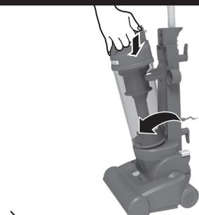
To remove the dust container from the cleaner, press the bin release button.
