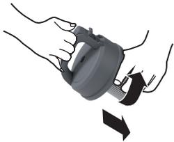
Hold the pre-motor filter, then rotate the bin lid with anti-clockwise direction.
