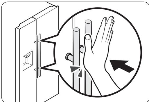
4. Firmly press the handles at the support. Check and make sure the handles are firmly attached.
