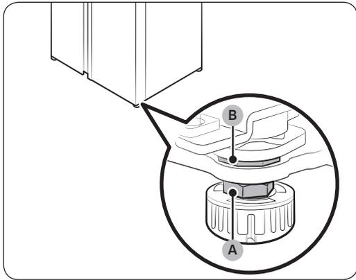
1. Open the door to adjust, and locate the two nuts (A) and (B) on the front bottom of the door.
