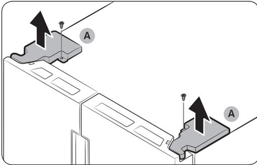
1. Use a Phillips screwdriver to unscrew the **hinge covers (A)** on the top of each door.
