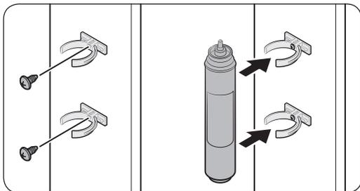
1. Attach the **lock clips** (x2) to appropriate positions under the sink, for instance. Then, fix the **lock clips** firmly using screws.
