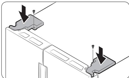
6. Insert the hinge covers with the front sides first, and then tighten the screws. Use a Phillips screwdriver for this step.
