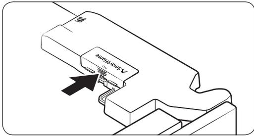
1. Press to unlock the arrow area of the adapter cover.
