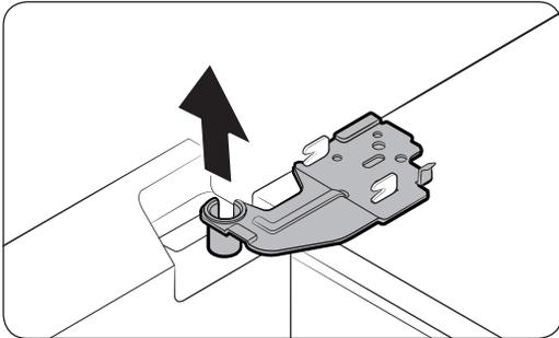
6. Open the door by 90 degrees. While holding the door, remove the hinge.
