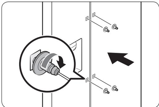
2. Use the Phillips screwdriver to assemble the fixers to the holes by tightening them clockwise.
