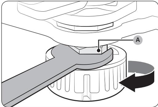
2. With a 19 mm spanner (not provided), turn the **clamp nut (A)** clockwise to loosen. Then, open the door, and do the following inside the door.
