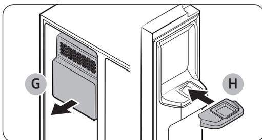
If you do not use the ice maker and need more storage space, remove the **icemaker bucket (G)**. Then, insert the **Freezer guide (Optional) (H)** on the ice chute.
