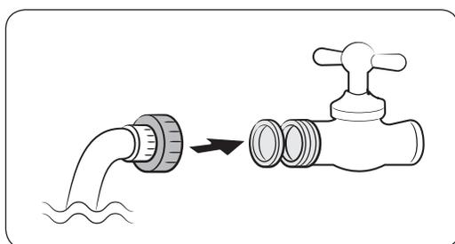
1. Assemble the water pipe line using couplers.
