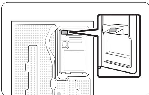
1. Open the door and locate the provided spacer.
