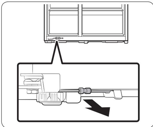
1. From the bottom rear side of the refrigerator, pull out the water line to the front.
