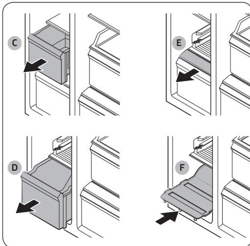
To secure more space, remove the **upper drawer (C)**, **lower drawer (D)**, and **lower drawer cover (E)**. Then, insert the provided **bottom shelf (F)**.
