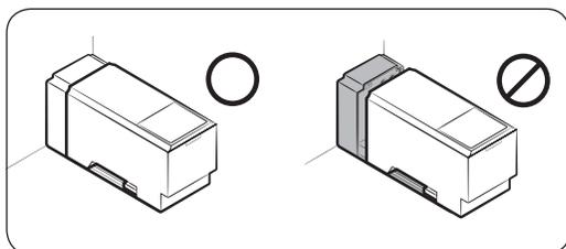
3. Reinsert the water tank and fit into the dispenser mechanism. Make sure the front side (with the front lid) of the tank faces to the front.
