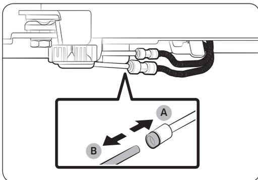
2. To disconnect the hoses, press and hold the **transparent coupler (A)** and detach the **water hose (B)**.
