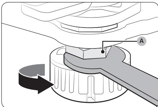
3. When complete, tighten the **clamp nut (A)** by turning it counter clockwise.
