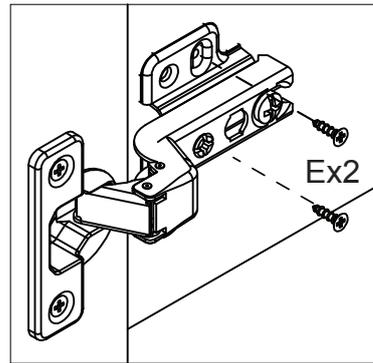
If it is necessary to re-align the door vertically, loosen the screws (X) and adjust the hinge plates up or down (Y) until gaps at top and bottom of the door are even, then re-tighten the screws.
