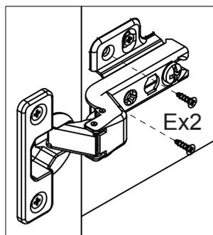
Once all the adjustments are complete and both doors are aligned, fix remaining x8 screws (E) into the other hinge plate holes then check all the other hinge screws are tight.
