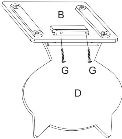
Secure Seat Back D to Seat B using 2 x Screw G.
