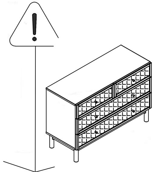
• A unit that is allowed to topple can cause serious or fatal injury. In addition to wall fixing the unit, place heavy items on the lower shelves, do not put any heavy objects on top of the unit and never allow children to climb or hang on drawers, doors or shelves.
