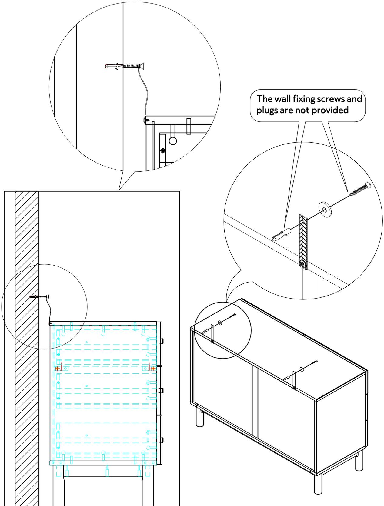
• **WARNING:** To prevent possible overbalancing this unit must be secured to a wall using the overbalance protector kit supplied.
