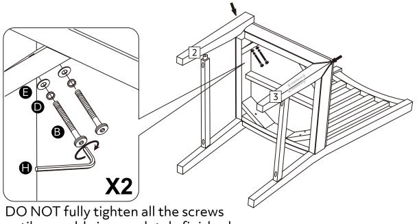
DO NOT fully tighten all the screws until assembly is completely finished
