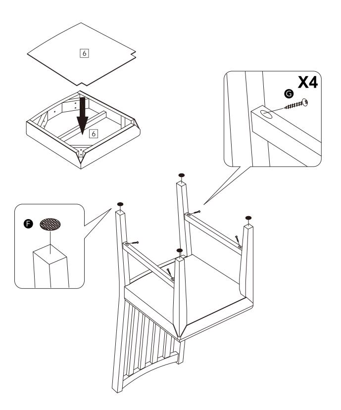
Fully tighten all the screws and bolts to complete assembly
