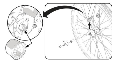
Take the front wheel and loosen the wheel nuts off each end of the axle. Remove the retaining washers from the axle.
