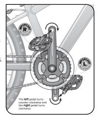
The spindle of each pedal is marked with an 'R' or 'L' corresponding to right and left respectively:
