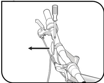
Position the white front reflector to the right of the handlebar stem so that it points directly forwards and is within 5 degrees of the vertical. Attach the bell in the same manner to the left of the handlebar stem.
