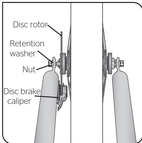
Slide the retaining washers onto the axle and ensure they lock into the forks.
