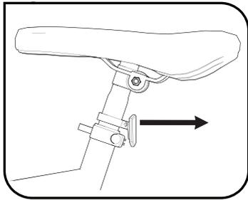
Position the red rear reflector on the seat post so that it points directly backwards and is within 5 degrees of the vertical.
