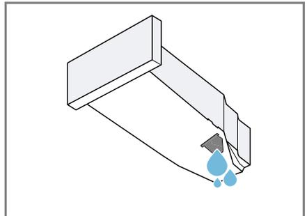
Check the condensation container filter → *Page 43* regularly and clean the filter if it is dirty. Make sure that you insert the condensation container before operating the appliance. → *"Inserting the condensation container", Page 34*
