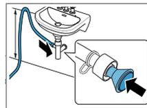
Secure the connection point with a (12-22 mm) hose clamp.
