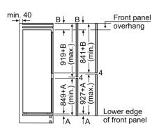
The specified unit door dimensions are valid for a door gap of 4 mm. measurements in mm
