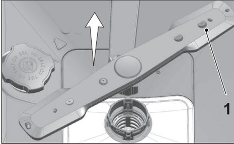
Check if the holes on the lower impeller assembly are clogged. If they are clogged, remove and clean the impeller assembly. (depends on model)
