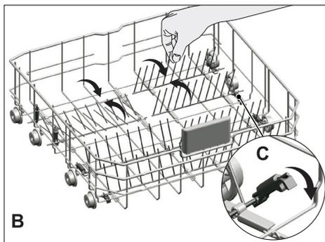
**i** Bringing the tines to the horizontal position by holding them from the tips may cause them to bend. Therefore, it will be appropriate to bring the tines in the middle to horizontal or vertical position by holding them from their stems and pushing in the direction of arrow.
