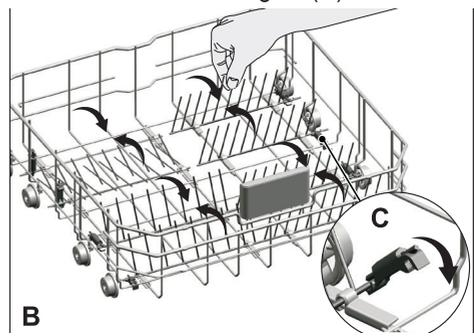
**i** Bringing the tines to the horizontal position by holding them from the tips may cause them to bend. Therefore, it will be appropriate to bring the tines in the middle to horizontal or vertical position by holding them from their stems and pushing in the direction of arrow.
