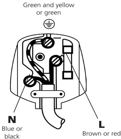
With the alternative plugs a 13A fuse must be fitted either in the plug or adaptor or in the main fuse box. If in doubt contact a qualified electrician.
