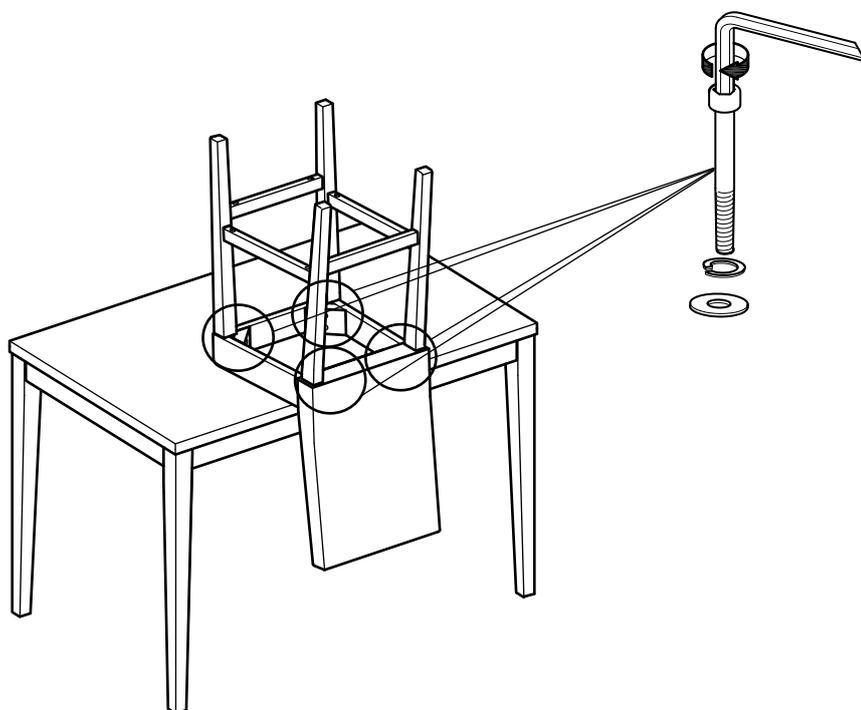
**d:** Highly recommend to re-tighten all the bolts again after using the chair for 7 days.
