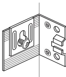
Fit the key-hole part of the Bracket over the screw, making sure that its protruding parts at the top and bottom are against the grooves in the Bracket
