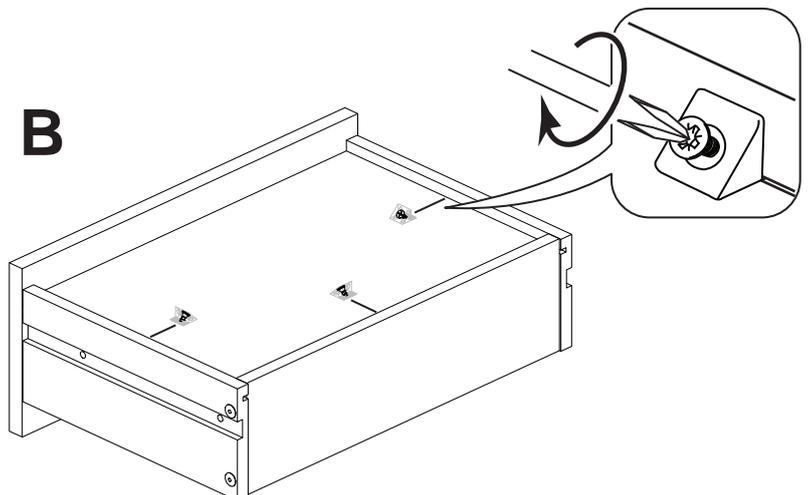
**Important:** Make sure that the drawer assembly is square before fitting the wedgefixes.
