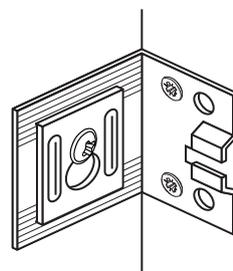
Make sure the unit is level, then drop the key-hole part over the Screw and tighten it up
