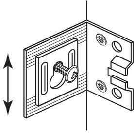
Loosen the screw in each Bracket and move the unit up or down.
