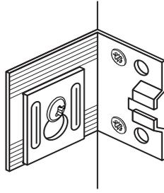
Drop the key-hole part back down over the screw and re-tighten it, making sure it locates into the grooves.
