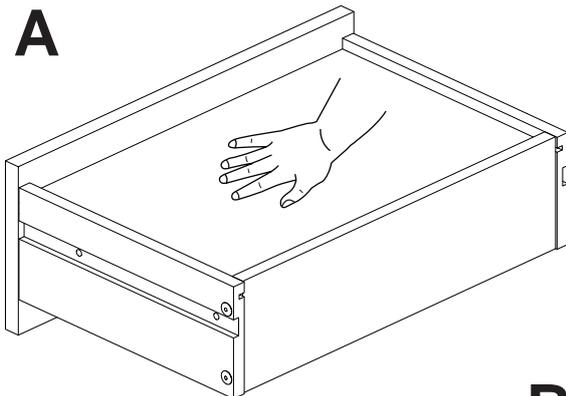
Make sure the Drawer Base panel is inserted in all 4 grooves. You may need to manoeuvre it slightly.
