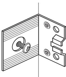
Carefully place the Bedside unit onto the wall by positioning the Brackets over the Screws
