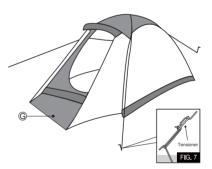
4. Insert the poles to the pin and ring(fig.4) and bend to fit the other end. Insert the arch pole on the eyelet, bend to he other end to fit the
