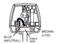
The wires in this mains lead are coloured in accordance with the following code:
