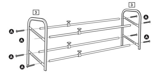
**b:** Set the width of the unit using the Tube clamps
