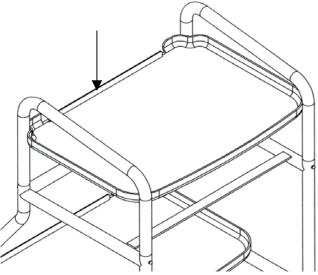
4. Insert the two trays on to the main frame. Slide the back of the tray on to the flat bar of the main frame then push down on the front of the tray (shown by arrow). Repeat for the other tray. (See diagram above).
