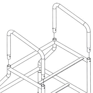
3. Insert the handle in to the top of the main frame. Hold in the brass push buttons on the handle whilst inserting. Insert the handle until the push buttons lock it in position. Repeat for the other handle. (See diagram above).
