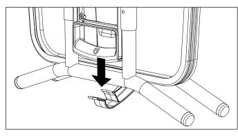
**4**. Secure the centre support strap by swinging it to the horizontal position and locating the notch over the protruding wires on the front leg.
