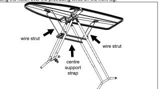
**5**. Rotate the wire struts to the position illustrated and gently push the ends of the wires into the moulded clips on the underside of the board.
