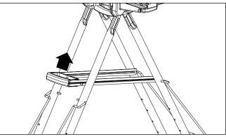
$10. \label{eq:10} \mbox{Continue to rotate the top and the front leg until the table returns to its folded position.}$
