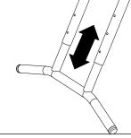
**4**. Repeat for the other leg mechanism – ensuring that both front and rear legs are adjusted to the same length.
