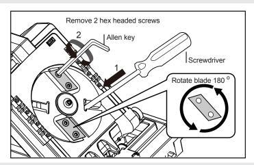
2. Since the blade is two side sharp for cutting, so could use both sides; Lock the blade disc using screwdriver or similar tools. Remove the blade by Allen key and rotate it through 180 degrees then fit the blade to the blade disc ensuring that the ground cutting edge is facing downwards; Fix the metal frame back with screws.
