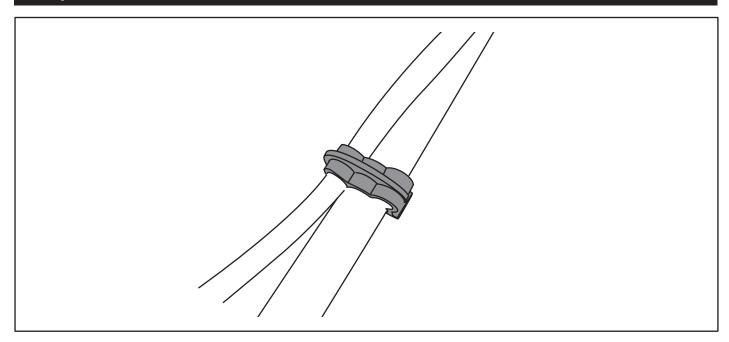
• Ensure that the cables clamps are used to fix the cable to the handle.
