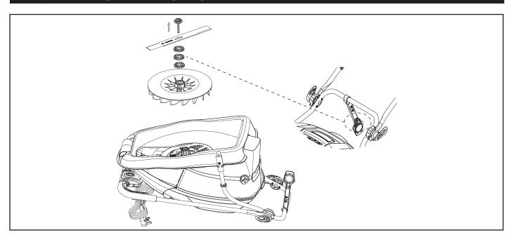
Remove the blade bolt by spanner provided, add a spacer between the blade and the impeller to reduce the cutting height 7mm.
