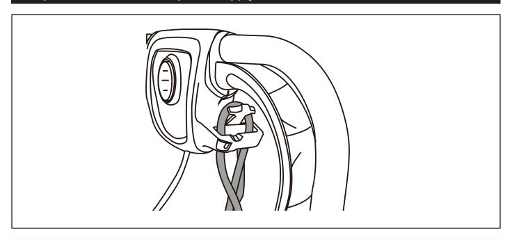
• Hook the mains cable through the cable strain-relief.
