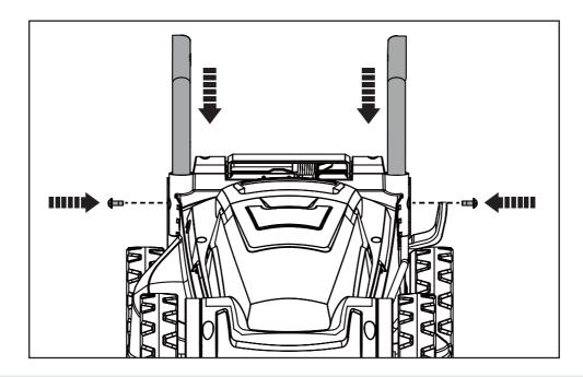
• Insert the Lower Handle Bar into the slot on the mower deck. Fasten in position with the 2 screws provided.
