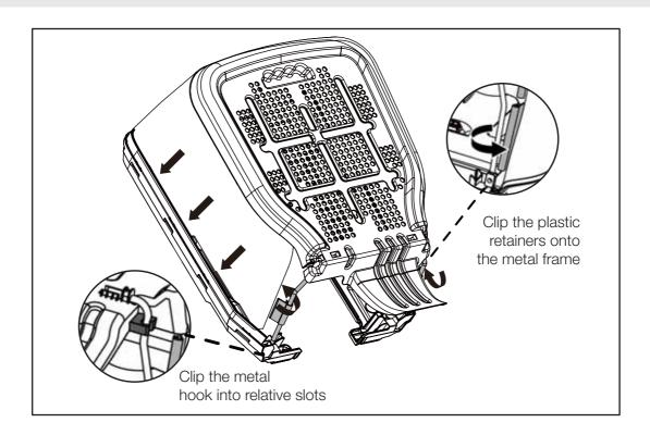
• Clip the plastic retainers onto the metal frame Ensure the side clamping sleeves are properly fixed on the frame.
