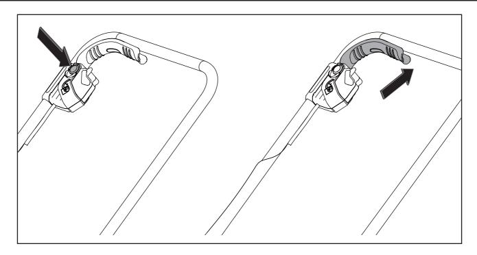
Press and hold the lock-off safety button to unlock the on/off lever then operate the on/off lever to switch the mower on. Release the on/off lever to off the mower.
