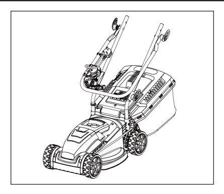
• When the two wing nuts are loosened, the handle can be folded for easy storage, Ensure the power cable is not caught between the folding sections.
