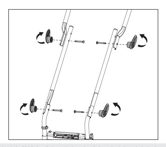
Attach the Middle handle bar to the lower handle bar using bolts and wingknobs.
