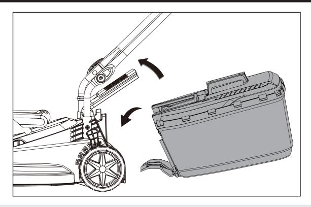
• Life the safety guard, then fit the grass bag onto the rear of the Mower, then release the safety guard. Ensure the safety guard fits firmly onto the grass bag.
