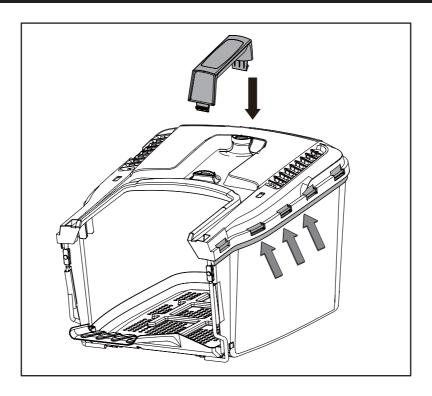
• Insert the collector handle into the grass bag, Clip the plastic retainers onto the metal frame.
