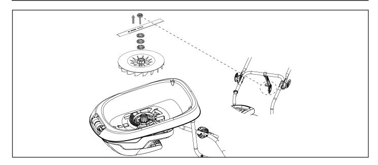
• Remove the blade bolt by spanner provided, add a spacer between the blade and the impeller to reduce the cutting height 7mm.
