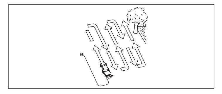
• To avoid cutting the mains cable and to collect grass clippings correctly please mow away from the plug socket following the arrows and avoid twisting the power cord.
