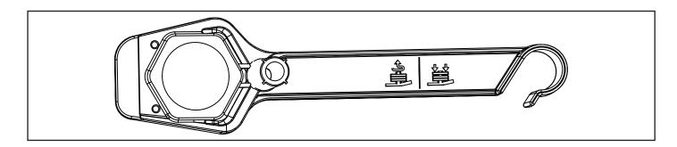
When removing a spacer from its storage location on the spanner, gently twist it as you remove it. When you replace a spacer back to this location just push it firmly into position.
