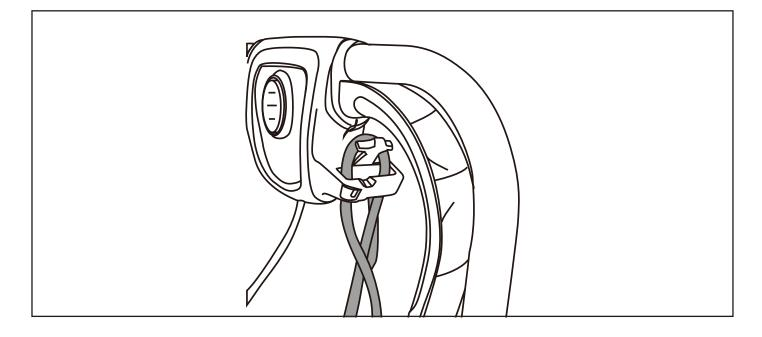
• Hook the mains cable through the cable strain-relief.
