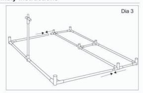
4. Insert the Long Tubes(4) into Joints(A) and Joints(B). Then insert the Short Tubes(5) into Joints(A) and Joints(B). See Dia 4.
