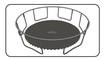
**Step 2**Attach the more circular end of the spring into one of the triangular rings on the mat. (see page 4 more details)
