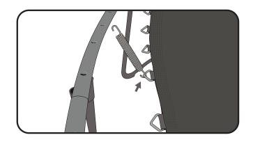
**Step 3**Then attach the other end of the spring to the frame.
