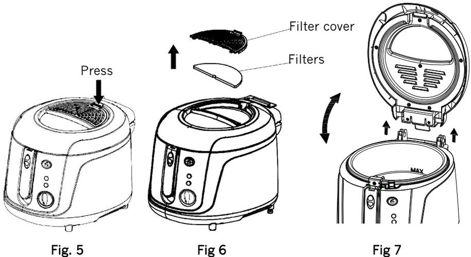
3. Open and remove the lid (fig. 7) and lift out the frying basket.
