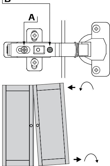
Adjusting the gap between the doors. Loosen screw 'A' slightly. Turn Screw 'B' clockwise to move the door away from the side, turn anti-clockwise to move the door towards the side. When gap is equal tighten screw 'A'.
