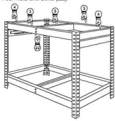
Fit the Right Hand Bracket with Roller Bearing Drawer Slide Attached (8). Leave two clear slots from the top as illustrated. Repeat this step for the Left Hand Bracket with Roller Bearing Slides (7). Fit the Centre Shelf Support (5) with the flat surface facing
