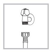
1. Connect the supply pipe by screwing it to a cold water tap using a <sup>3</sup>/<sub>4</sub> gas threaded connection (see figure).
