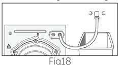
**2:**The straight connection attaches to the water supply valve.(Fig 19)
