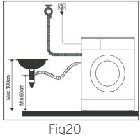
Drain hose can be fitted to the drainer or a wash basin.
