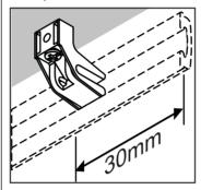
6. Slide or clip the rail onto the mounted brackets.
