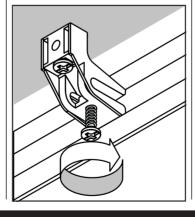
8. Clean the ends of the rail and fit an end stop at each end of the rail. Turn the locking screws to secure the ends in the rail.
