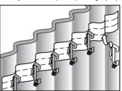
10. Engage the bottom of the Glidehooks with the bottom of the rail and snap top of Glidehooks over the top of the rail and Ensure end Glidehooks are snapped into end stops.
