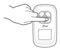
Press the button and hold for two seconds to turn the Parent unit on.
