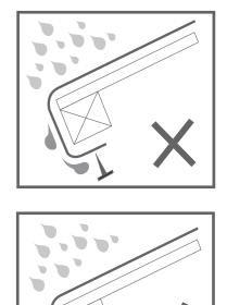
Fix the trims to each corner of the building and across the joint at the back, securing each trim into place with 3x30mm screws
