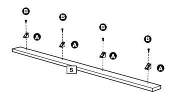
**b:** Use Screws **3** to fix the Front panel **5** onto the Bottom panel **2**.
