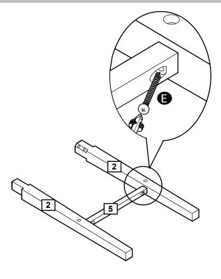
**b:** Attach legs 2 to front corners of the seat frame. Use bolts A with spring washers 3 and washers 6 into each 2 holes in the front corners. Tighten bolts with allen key 6.
