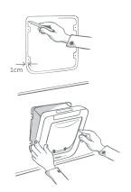
If there is metal present you will need to cut a larger hole in your door, leaving a gap of 2-3cm (1-1.2") between the tunnel of the pet door and the metal in your door. To begin with, trace around the outer edge of the back frame as a size guide. Now mark your cutting line 1cm (0.3") inside the line you have traced around the back frame, leaving the screw holes in place. Cut this hole and reinstall the pet door.
