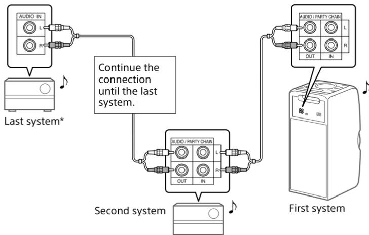
\* Connect the system which is not equipped with the Party Chain function at the last system. Be sure to select the Audio In function on this last system.
