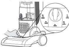
Ensure that the cleaner is in the upright (parked) position and move the selector to the required setting for the carpet type or floor covering.
