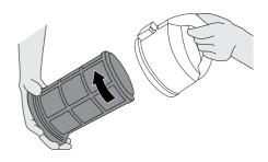
Wash both filter and protective mesh under warm water until the water runs clean. Remove excess water by shaking and leave to dry for 24 hours. Reassemble and refit filters to cleaner, only when they are completely dry.
