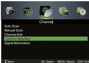
3. A Common Interface main menu will pop up. Press the **▲▼** buttons to select the items and press the **OK** button to confirm.
