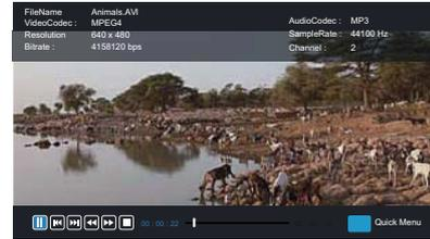
6. Press the **OK** button or the **DISPLAY** button to display the function bar. Press the buttons and then press the **OK** button to select the function: Pause / Prev. / Next / FB / FF / Stop / Quick Menu (Repeat / Encode Type).
