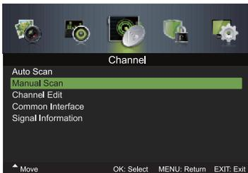
2. Press the **▲▼** buttons to select **Manual Scan** and then press the **OK** button. On the submenu, select Digital Manual Scan and then press the **OK** button.
