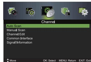
2. Press the **▲▼** buttons to select Auto Scan and then press the **OK** button to enter submenu.
