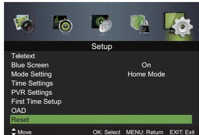
3. Press the **▲▼** buttons to select Yes or No on the screen. All settings will be reset to factory defaults and the Setup menu will disappear.
