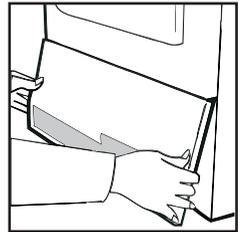
2. Pull firmly on the handgrip and slide the water container out of the dryer.
