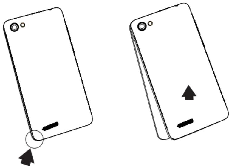
Lift the back cover using the notch
