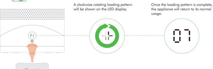
When you have re-assembled your appliance, press and hold the 'Standby ON/OFF' button for 6 seconds on the remote control to reset the filter indicator.
