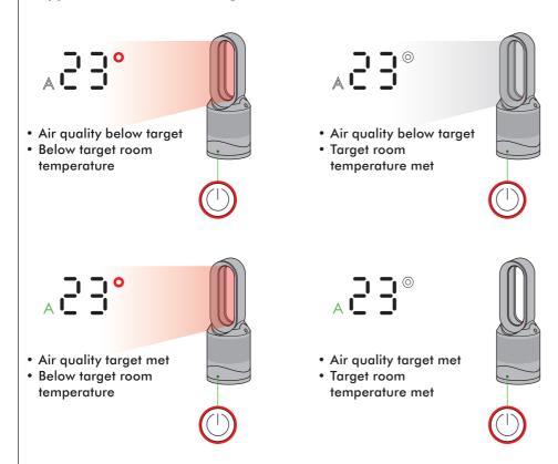
When auto mode is used while in heating mode, the appliance is both purifying and heating the air. The appliance will display the target room temperature, not the fan airflow. Once the target room temperature has been reached, the appliance will stop heating the air. If the air quality target has not been met, the fan will continue to run in order to keep purifying the air. If the room temperature falls below the target temperature, the appliance will start to heat again.
