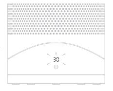
To set the sleep timer, select the desired time. When time reaches zero, the appliance will go into standby mode. To cancel, increase the time until two dashes appear.
